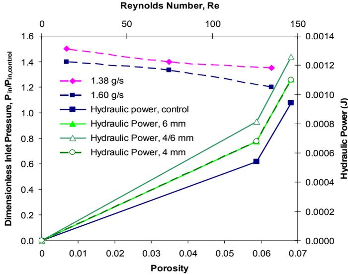
**Figure 8: Calculated Dimensionless Inlet Pressure and Hydraulic Power at Different Porosities and Reynolds Number, respectively**
