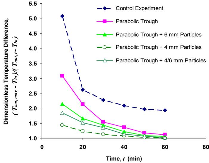
**Figure 4: Calculated Dimensionless Temperature Difference for Different Arrangements of Solar Heating Panels performing hydrostatically: The Time Response of the Solar Collector**
