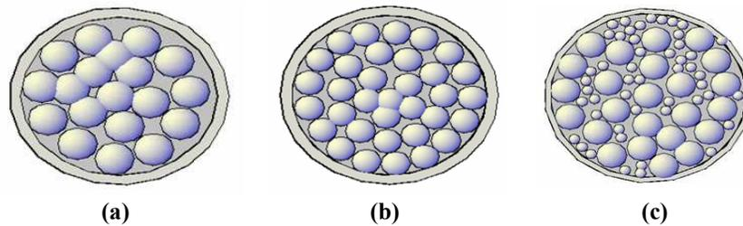
**Figure 2: Schematic Diagram showing the Current Porous Medium within the Steel Pipes: (a) 6 mm diameter, (b) 4 mm diameter, and (c) mixed between 4 and 6 mm Spherical Particles**
