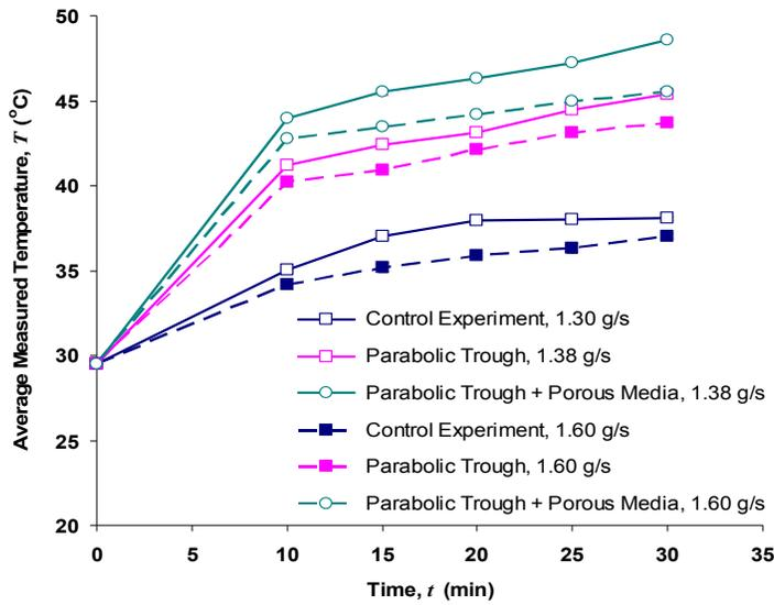
**Figure 5: Measured Outlet Water Temperature Distributions for Solar Collectors running hydrodynamically, A Porosity of 0.0068 is selected in the Porous Media Heat Transfer Study**
