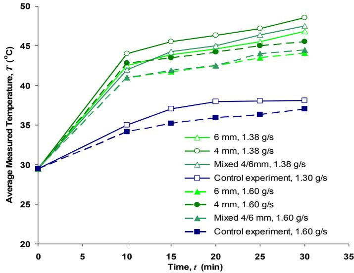
**Figure 6: Measured Outlet Water Temperature Distributions at Different Porosities and Mass Flow Rates**
