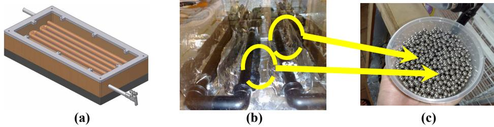
**Figure 1(a): Schematic Drawing of the Current Solar Heat Panel; (b) Solar Heating Panel with a PTC installed; and (c) Mild Steel Particles used in the Study**
