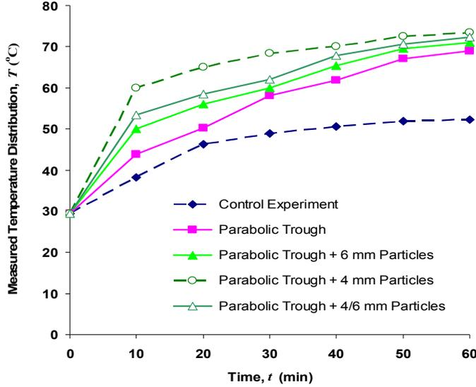
**Figure 3: Measured Outlet Water Temperature Distributions for Different Arrangements of Solar Heating Panels performing hydrostatically**
