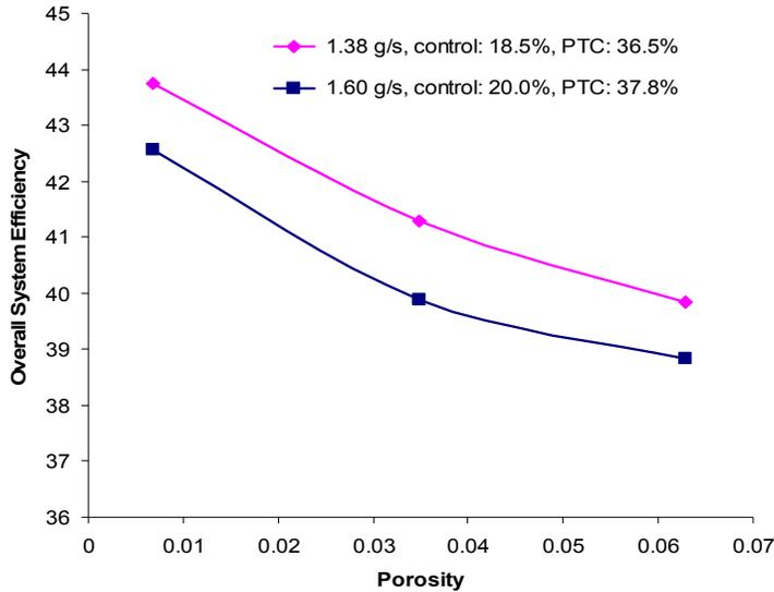
**Figure 9: Calculated Overall System Efficiency at Different Porosities and Mass Flow Rate**
