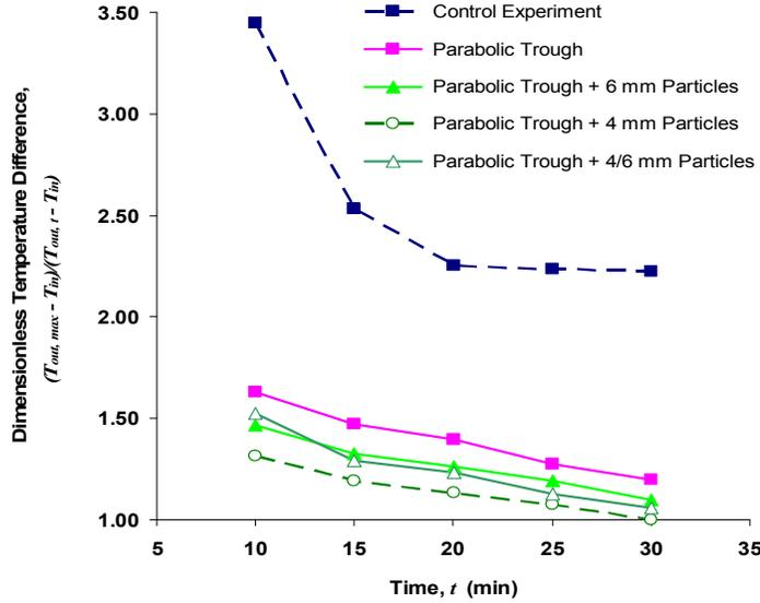
**Figure 7: Calculated Dimensionless Temperature Difference for Solar Collectors performing hydrodynamically: The Time Response of a Solar Heat Panel at  $Re = 126$**
