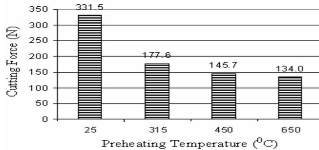
Figure 6: Effect of Preheating on Cutting Force ( $V=70$  m./min,  $d=1$  mm, Feed = 0.088 mm/tooth)
