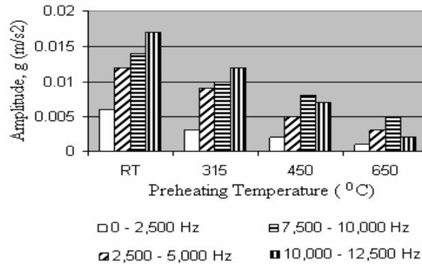
**Figure 8: Effect of Preheating Temperature on Acceleration Amplitude of Vibration (inserts: uncoated WC-Co)**
