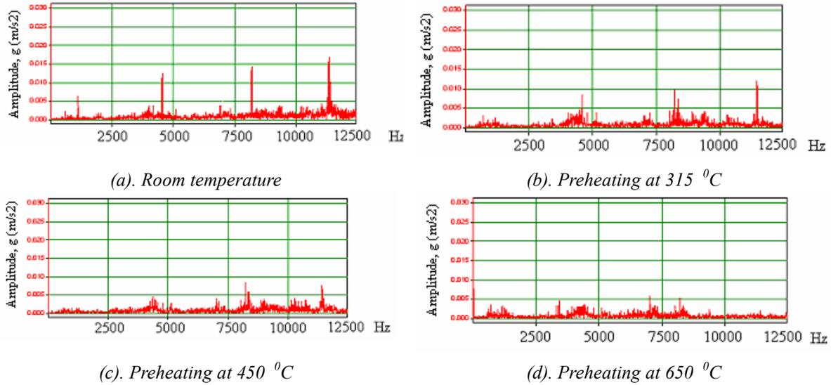
**Figure 7: FFT Output of End Milling (Cutting speed: 70 m/min, axial depth of cut: 1 mm, feed: 0.088 mm/tooth)**
