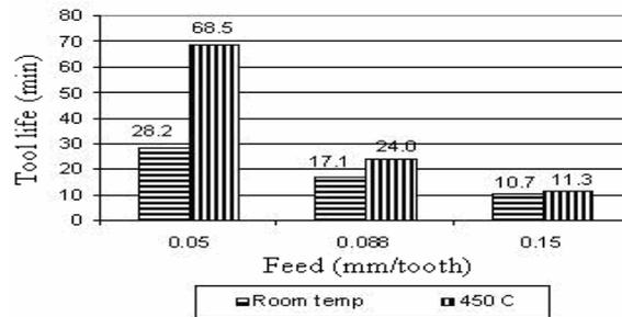
**Figure 4: Effects of Feed on Tool Life (V=70 m/min, axial DOC = 1 mm)**
