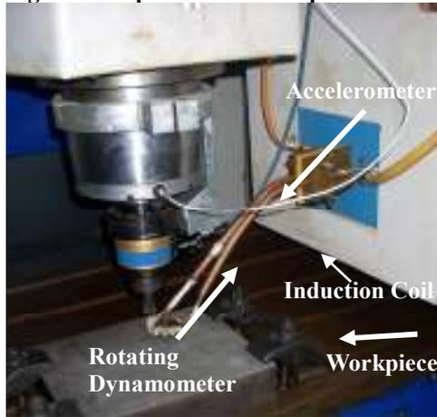
The experimental set up for the machining is presented in Figure 1. Flank wear has been considered as the criteria for tool failure and the wear was measured under a Hisomet II Toolmaker's microscope. Tool life experiments were stopped when an average flank wear achieved exceeded 0.3 mm.
