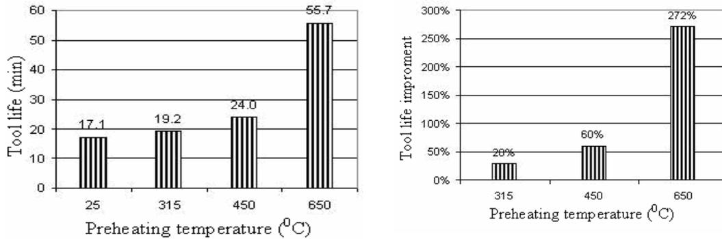
(a). Tool life vs Preheating Temperature (b). Tool life improvement vs Preheating temperature
