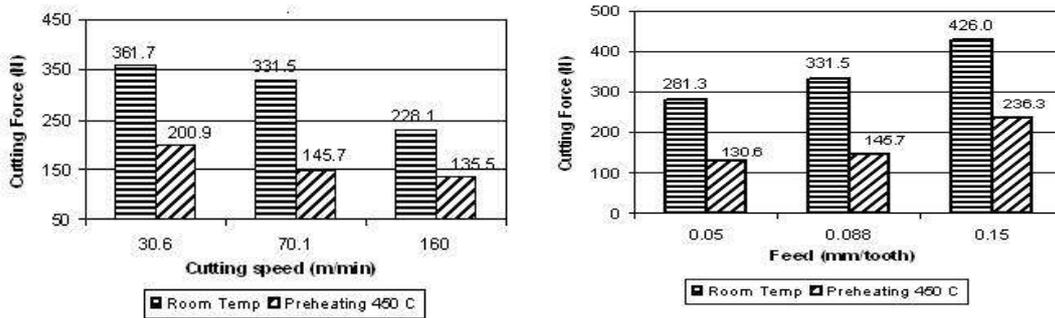
(a). Cutting Force vs Cutting speed
