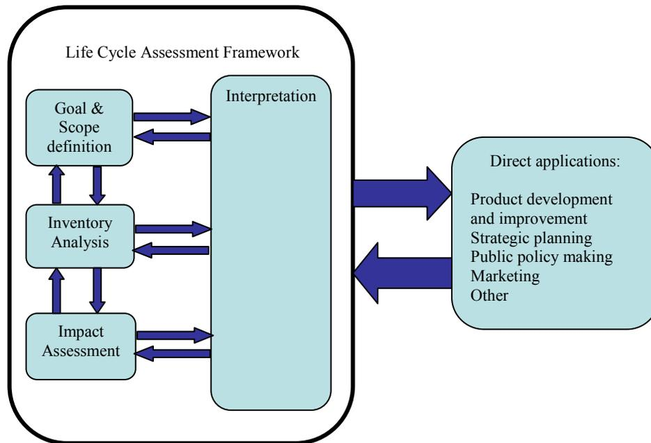
Figure 12: Phase of an LCA. Source: ISO 14040 (1997)
